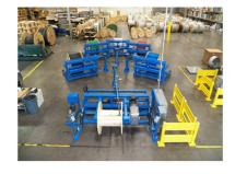
With our high speed paralleling machine that spools the wires onto the reel all at the same time
